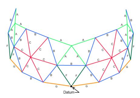
Figure 7 - Adding cross struts in A-B-A pattern.
