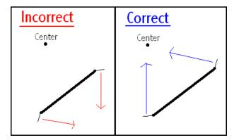
Figure 2 – Attention: The bent edges of each strut must be placed towards the center of the dome or the dome will not fit together.
