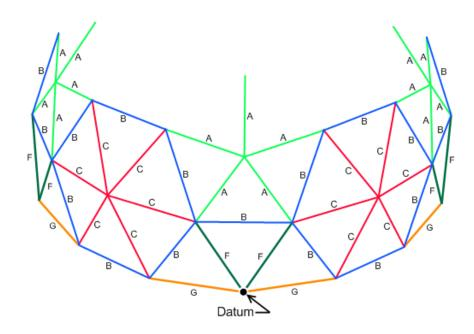
Figure 8 - Add 5 A's to the structure.
