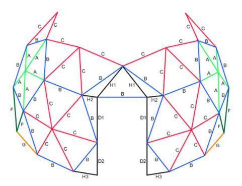
Figure 13 – Install the doorway struts.
