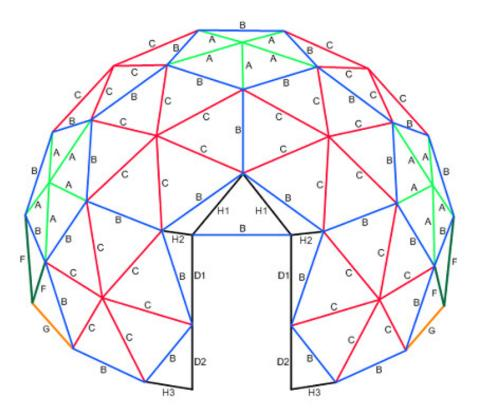
Figure 17 – Adding Vertical B struts.
