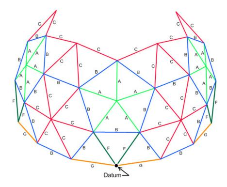
Figure 10 - Attach cross struts (All C's).
