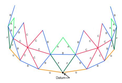
Figure 6 - Adding zigzag row (A-B-C-C-B-A pattern)
