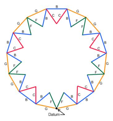
Figure 3 - F-B-C-C-B-F zigzag pattern along bottom row.
