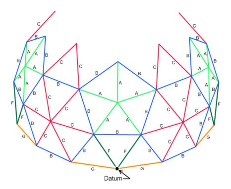
Figure 9 - Completing pentagons and adding triangles to cross struts.
