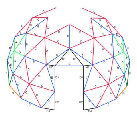
Figure 15 – Install 10 C struts.
