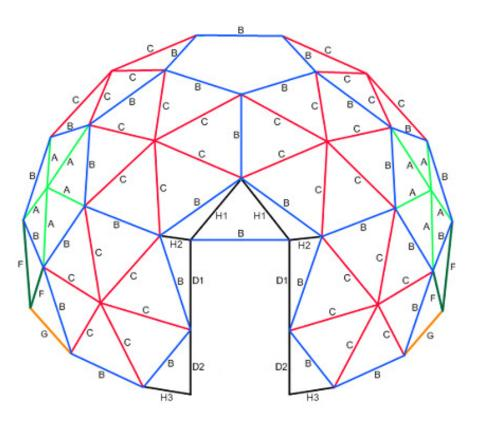
Figure 16 – Install 5 B struts.
