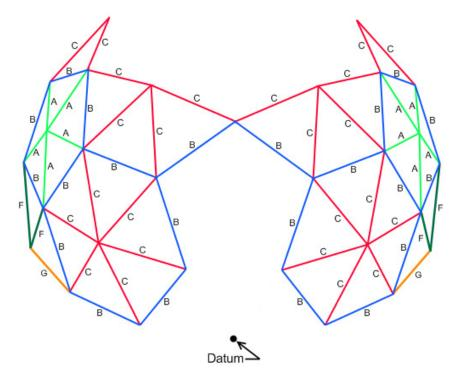
Figure 12 - Remove B-F-F triangle and G struts.
